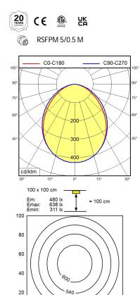
Light sourceLEDWork equipmentWithoutConnected load22 - 26 V; DCPower consumptionca. 24 W
